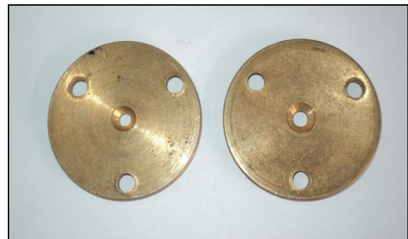
Orifice plate of Dia 5 mm & 6 mm
