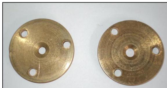
Orifice plate of Dia 5 mm & 6 mm
